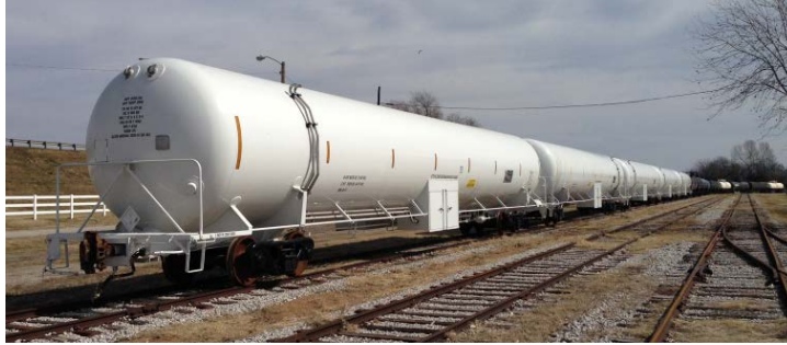
DOT-113C120W Tank Car. ~30,000 gallons net volume
