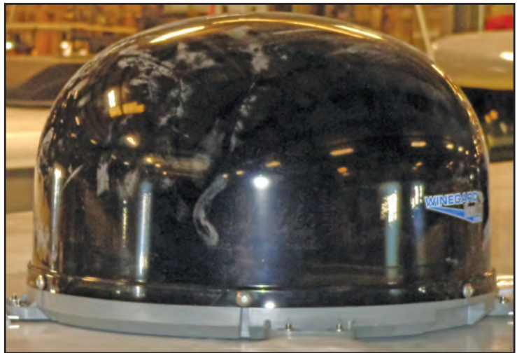
Figure 6-1: The dome satellite on top of the motorhome can be raised allowing easy access to change dip switches to a new satellite provider.
