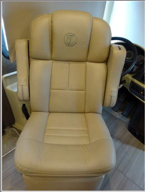
Figure 7-4: Both the driver's and passenger's chairs swivel to face the living area of the coach
