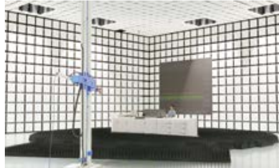
EMI measurement of products in a semi-anechoic chamber
