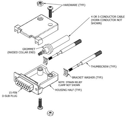
Figure 20 Harness Plug Assembly
