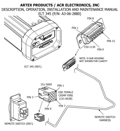
Figure 19 Remote Switch Harness Arrangement
