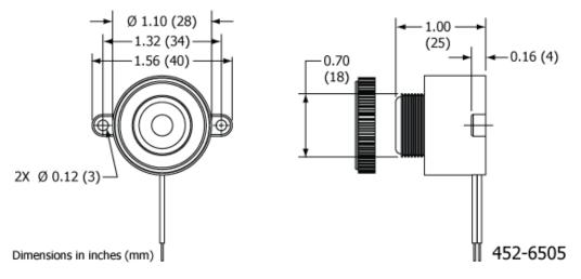
**Figure 16 Buzzer Outline and Dimensions**
