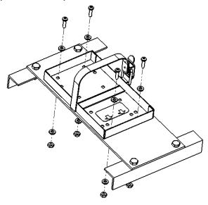
Figure 13 Typical Mounting Tray Installation
