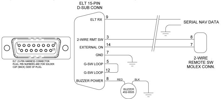
Figure 17 Typical 2-Wire Installation for Unshielded Harness
