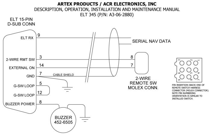
Figure 18 Typical 2-Wire Installation for Shielded Harness
