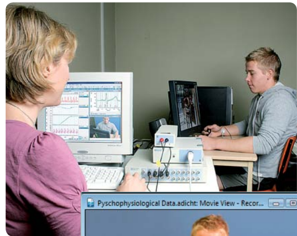
A recording of data from a human subject during stimulus presentation. Data acquired include finger pulse, EOG, GSR, ECG and EEG.
