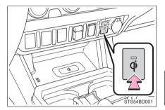
Place a mobile device on the tray as shown in the illustration.
