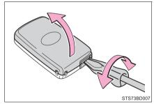
Remove the depleted battery.
