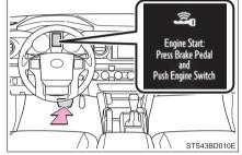
Press the engine switch shortly and firmly.
