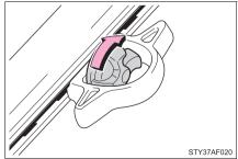
5 Check the tie-down cleat to confirm that it is locked into a detent and securely mounted to the deck rail system.
