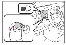
2 Press the Automatic High Beam switch.
