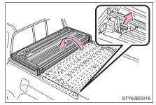
4 Secure by using the storage straps.
