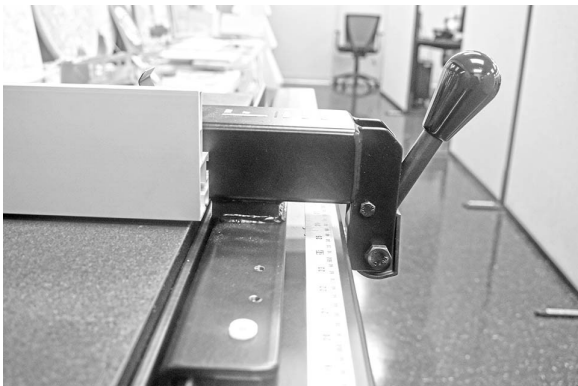
Fence fitted over the front guide rail
