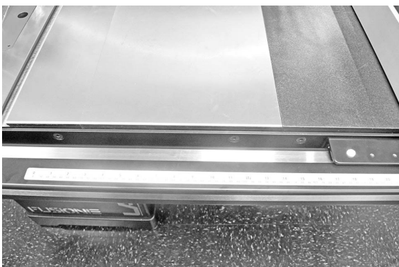
Front of rail showing counter sunk screws
