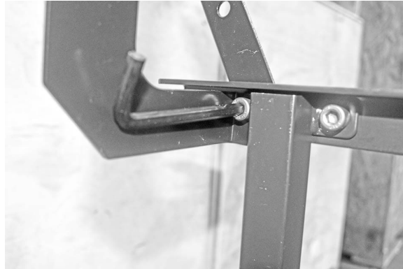
Hose support and Leg properly Installed:
