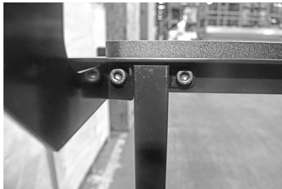
Hose support and Leg properly Installed:
