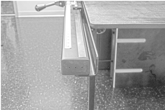
Front guide rail seated on front rail:
