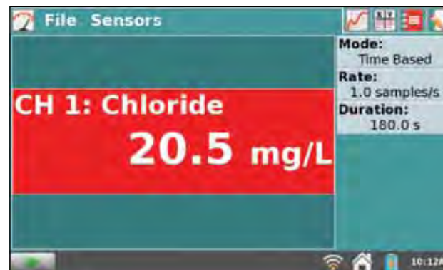
Testing the chloride ion concentration of pond water
