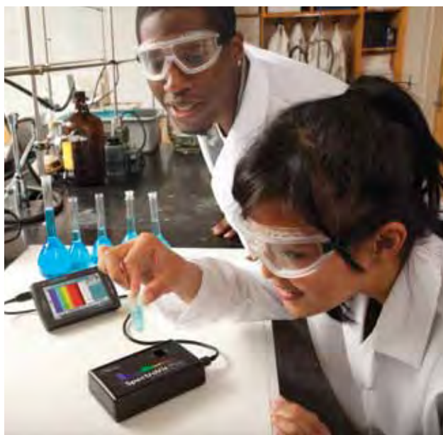
Examining the absorbance spectrum of copper (II) sulfate using SpectroVis Plus and LabQuest 2
