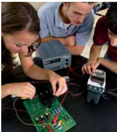
Studying Ohm's law using the Current Probe, Differential Voltage Probe, and the Vernier Circuit Board
