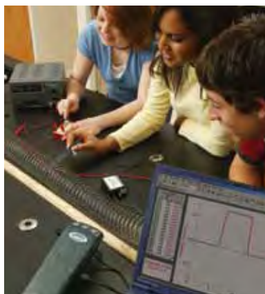
Measuring the magnetic field in a coil
