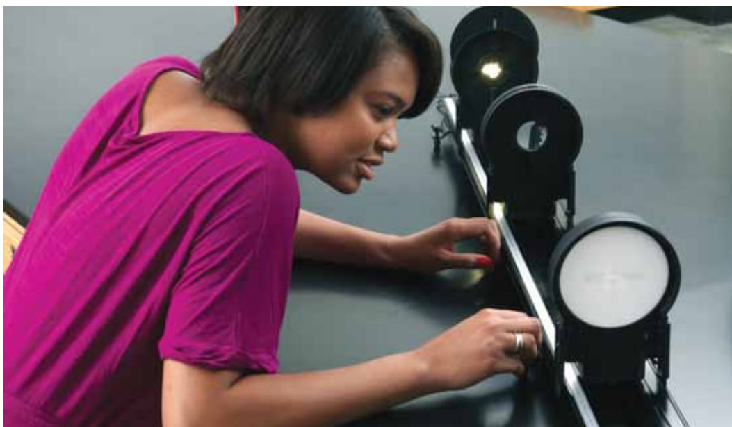
Viewing an inverted image using a single thin lens from the Optics Expansion Kit mounted on the Vernier Dynamics System track
