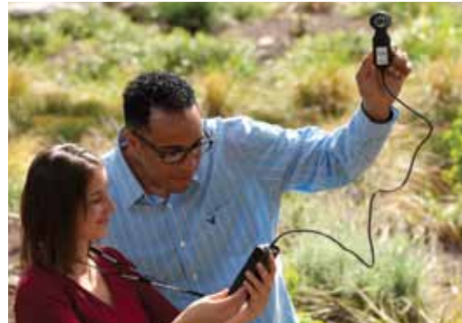
Using the Anemometer to measure wind speed
