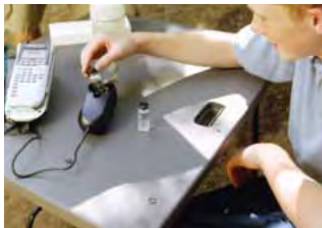
Measuring turbidity of a stream sample
