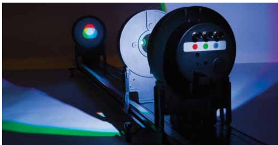
Mixing equal intensities of red, blue, and green to get white light
