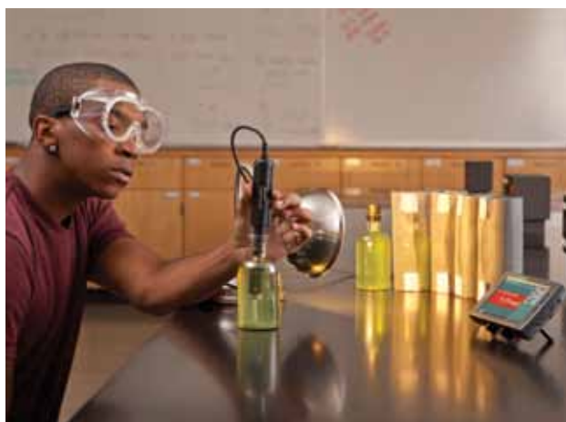
Using the Vernier Optical DO Probe to measure primary productivity
