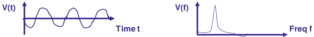
Fig. 4- Example of Narrowband Ingress Noise in the Time Domain and Frequency Domain
