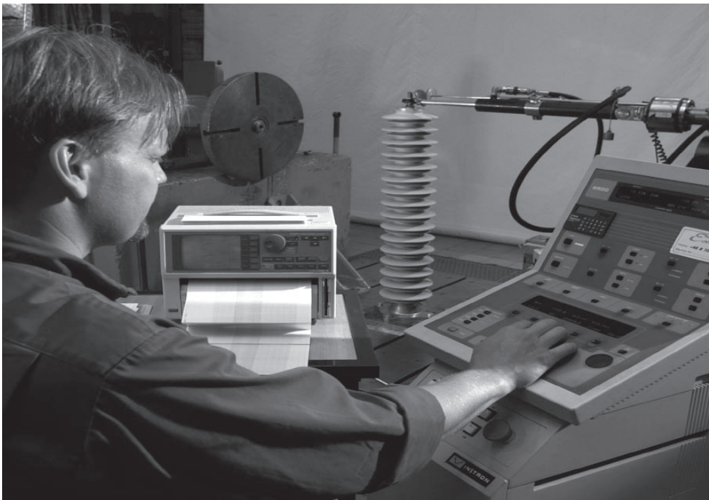
Mechanical test of silicocone-housed arrester PEXLIM P.
