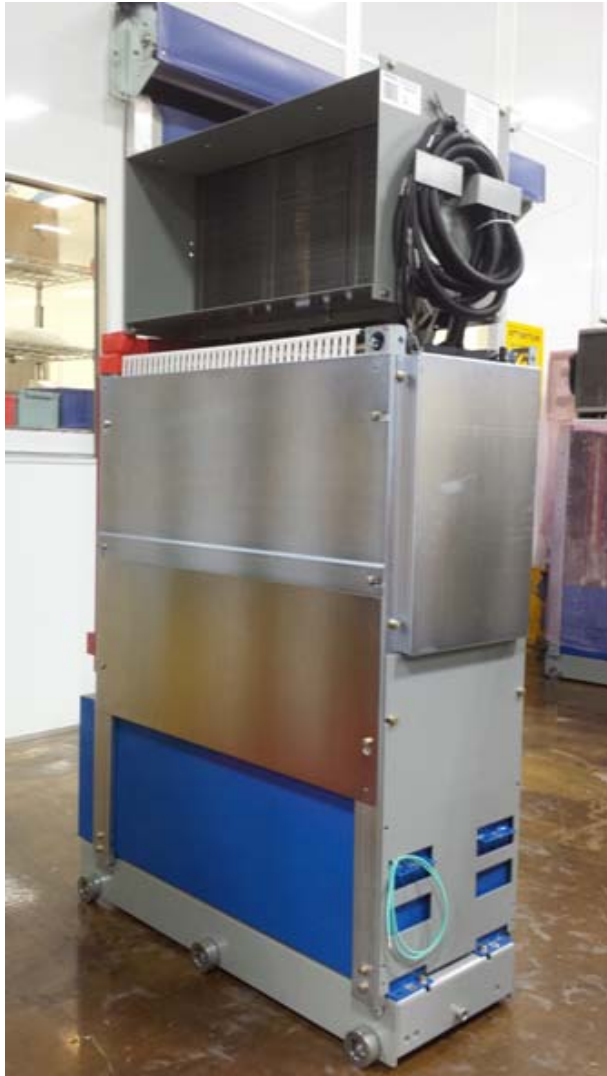
Figure 14. 1250 hp three-phase EP inverter
