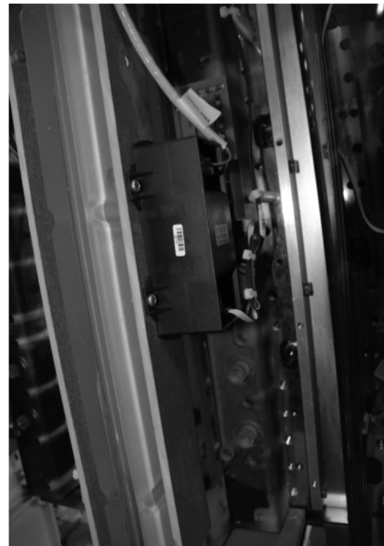
Figure 35. Mount paddles with power supplies and gate drivers (IMPORTANT: Remove bonding and use static precautions)
