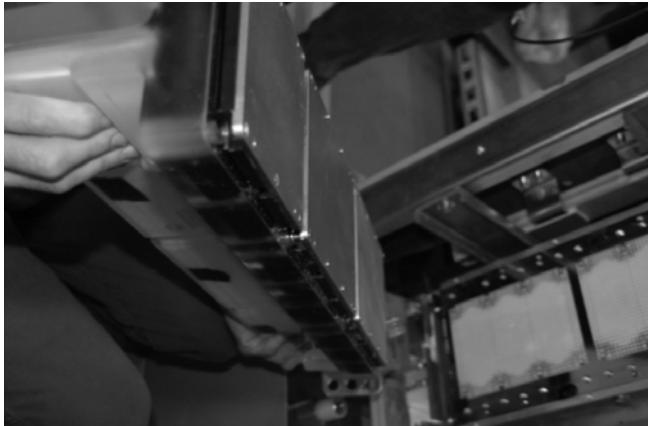
Figure 32. Place power pole on heatpipe
