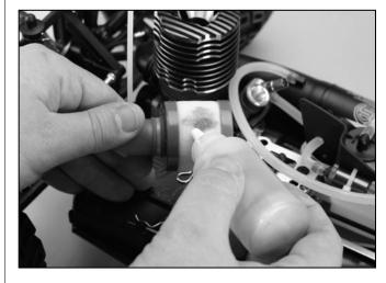
**Step #6**Apply air filter oil (not included) and spread the oil uniformly onto the air filter allowing it to saturate the foam element.
