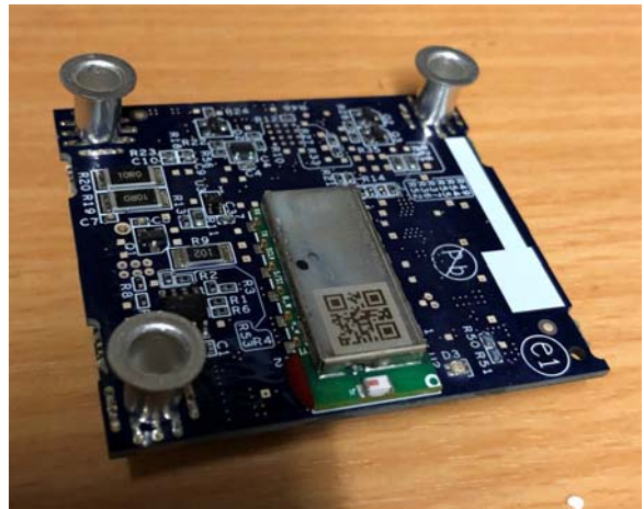
Fig. 25 – Bluetooth Module (used on all models)
