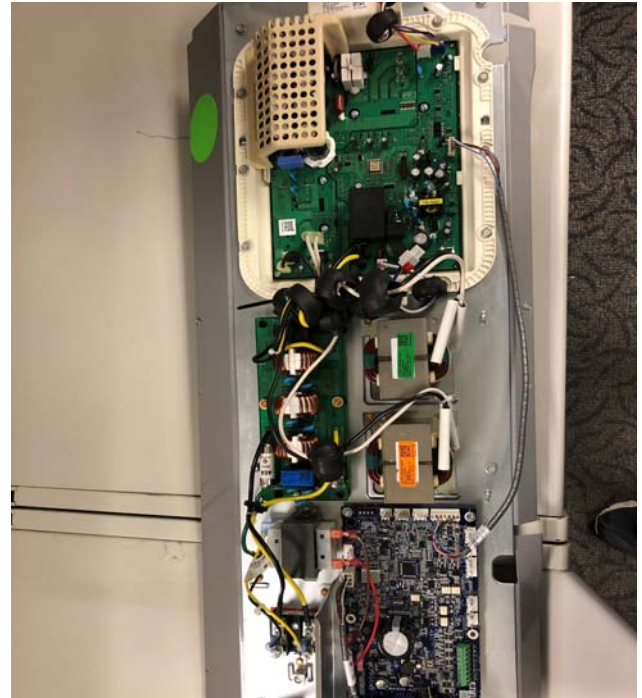
Fig. 19 – 4T/5T Control Box
