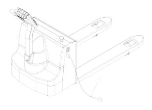
• Installation is in the reverse order of operations, pay attention on battery install position and cable connection. Make sure the well place cables to avoid be damaged when you removal and installation battery.
