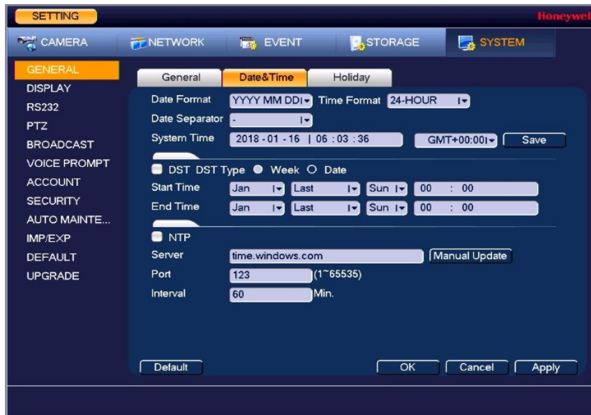
Figure 10-2 Date and Time Configuration Tab
