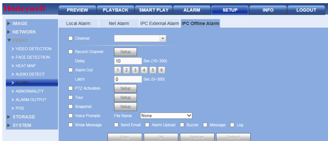
Figure 12-74 WEB - IPC Offline Alarm Configuration Interface
