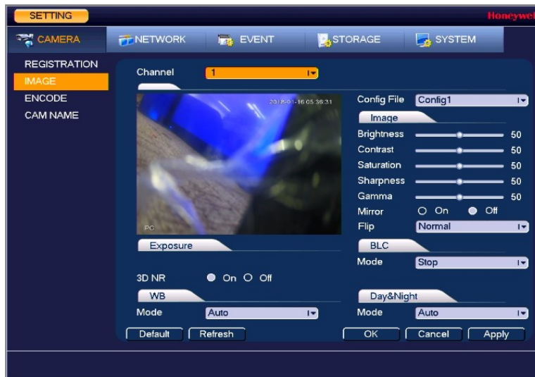
Figure 6-2 Camera Image Settings Tab
