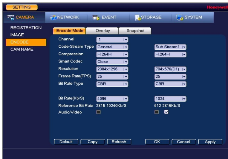
Figure 6-4 Camera Encoding Settings Tab
