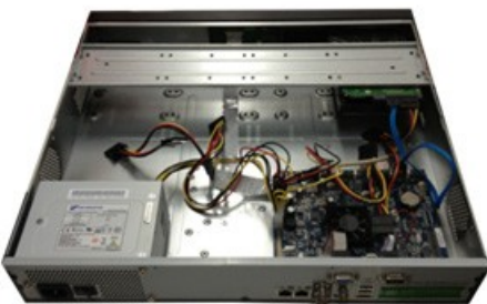
Figure 15-11 Connecting the HDD and the Power Cable
