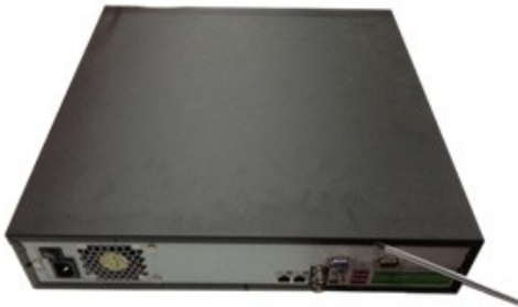
Figure 15-13 Removing the NVR Cover
