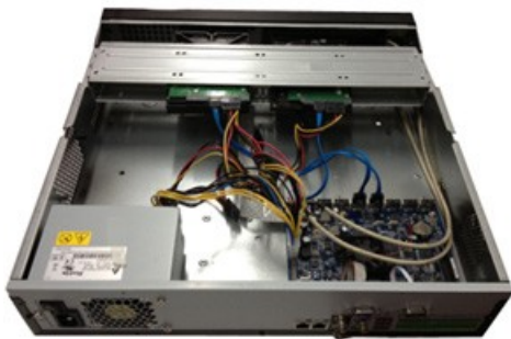
Figure 15-16 Connecting the HDD and the Power Cable
