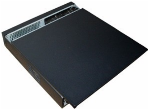
Figure 15-12 Replacing the NVR Cover
