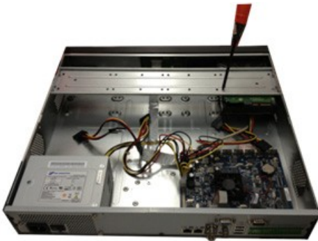
Figure 15-10 Placing the HDD
