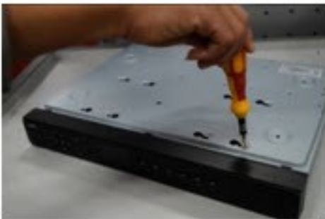
Figure 15-4 Securing the HDD to the NVR Housing
