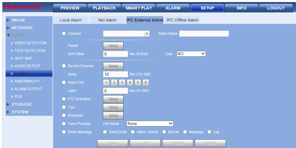
Figure 12-73 WEB - IPC External Alarm Configuration Interface
