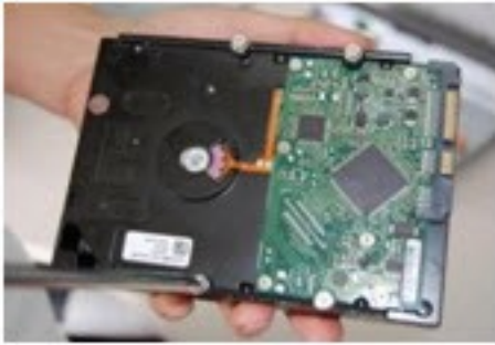
Figure 15-9 Loosening the Four Screws in the HDD Housing
