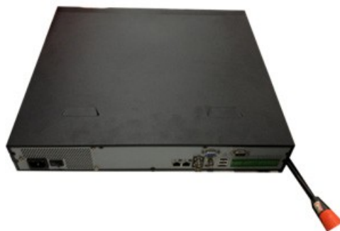
Figure 15-8 Removing the NVR Cover
