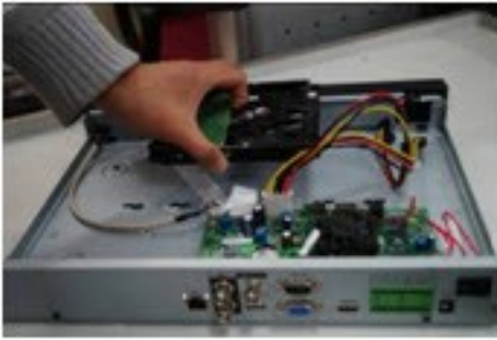
Figure 15-3 Placing the HDD
