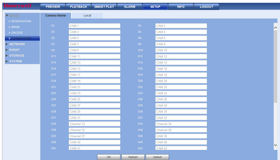
Figure 12-35 Camera Name Configuration Interface
