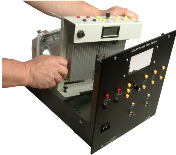
Figure 32. Installing a solar panel in the Solar Panel Test Bench.
