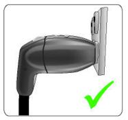
3. With your vehicle unlocked, press the button on the top of the Mobile Connector. The charge port door opens.
