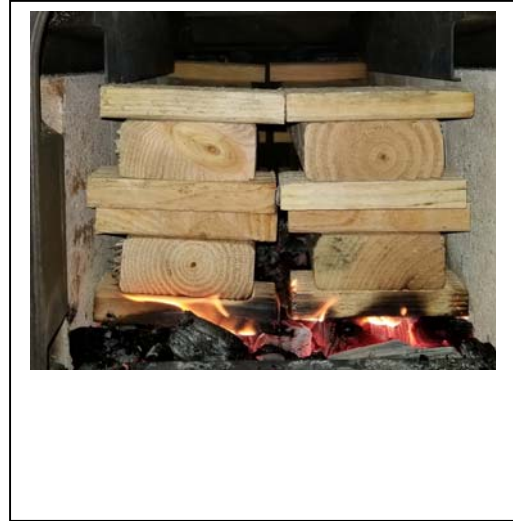
Run 3 – Newly Loaded Stove
