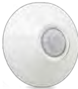
Ceiling-mount Sensors: The nCM 10 passive infrared sensor is the best choice for detecting walking motions in hallways. Provides 28 ft. radial coverage when mounted to a standard 9 ft. ceiling height. 360 degree coverage pattern detects occupants immediately upon entrance to hallway.
