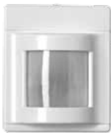
Hallway Sensors: Designed for 7-10 ft. mounting at end of hallways. Sensors should always be applied in pairs facing each other.
