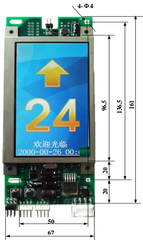
Diagram 3-22 BL2000-HEH-L2.3 Appearance and layout installation dimension
