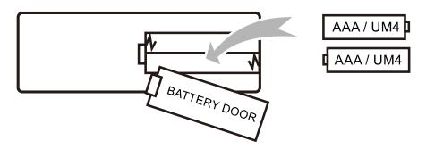
Remove the battery compartment cover on the back of your remote by carefully sliding to open. The battery cover can then be lifted away. Fit the correct batteries (2XAAA batteries not included ), referring to the polarity markings. Finally, replace the cover.
