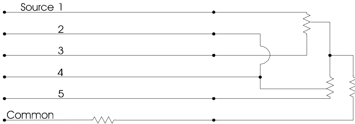
Figure 5-2. Field-wired Circuit with a Common Return
