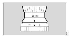
1 Turn the APL valve head counterclockwise to its final position stop.
