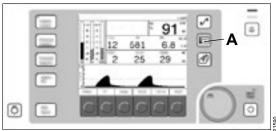
The volume alarms can be switched on and off during operation by pressing the key (A), see chapter "Switching the volume alarms on and off" on page 145.
