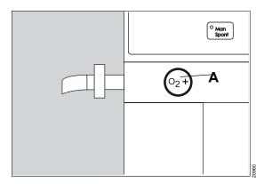
The O2 flush is used for flushing and quickly filling the breathing system and breathing bag with O2 while bypassing the vaporizer.
