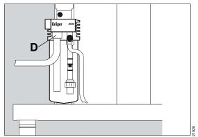
4 If necessary, connect the anesthetic gas scavenging hose of the non-rebreathing system to the second connection (D) of the anesthetic gas receiving system.
