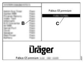
The test results (B) are displayed on the screen. After completion of the system test, the total test results (C) are displayed, see chapter "Checking the readiness for operation" on page 87. If the system test was successful, the *Standby* mode is activated.
