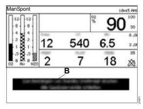
The pressure waveform window is replaced by a confirmation message (B) and instructions to turn off the flow.
