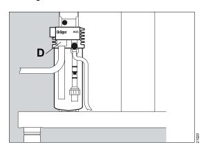
3 If necessary, connect the non-rebreathing system scavenging hose to the second connection (D) of the anesthetic gas receiving system.
