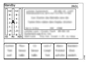
If the standard resolution is configured, the electronic fresh-gas flow displays show the flow in increments of 100 mL/min (format xx.x L/min). The virtual flow tubes (A) of the screen indicate a range from 0 to 12 L/min.
