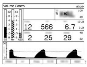
During the calibration, the O2 value in the window (B) of the O2 monitoring is replaced by the word *CAL*. The calibration time is approx. 15 seconds. After successful calibration, the O2 measured value is again displayed.
