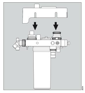
1 Fit the COSY cover to the breathing system, taking care that all cables are passed through the openings provided.
