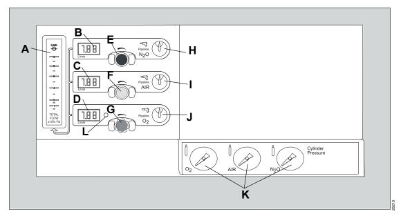
The total flow tube and the pressure gauge are located on the front of the device below the screen.
