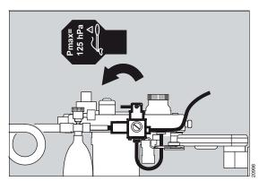
Diverting the fresh-gas flow to the non-rebreathing system:
