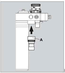
Screw on the exhaust port (A) in the compact breathing system from below.
