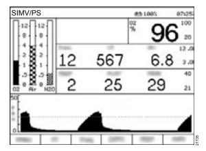
In the following table, all parameters (B) in **SIMV/PS** mode, together with the corresponding setting ranges and factory settings, are listed.
