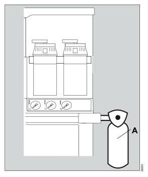
1 Hang the completely prepared and functionally checked manual resuscitator (A) to the right on the transport rail.
