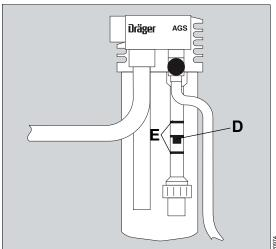
The top edge of the float (D) in the flow tube must move between the two marks (E).
