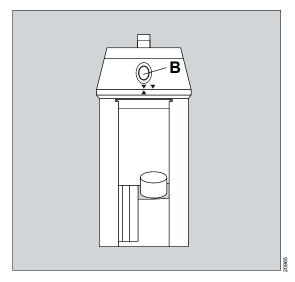
2 Set the control dial (B) of the vaporizer until it engages on 0.
