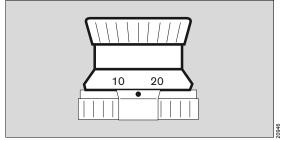
1 Set the APL valve head to the desired maximum airway pressure.
