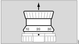
In the *ManSpont* mode, lifting the valve head relieves pressure from the breathing system.
