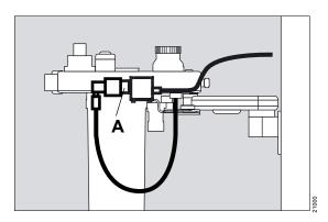
1 Remove fresh-gas hose from the external fresh-gas outlet (A).
