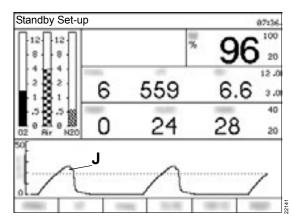
When the setting **Normal** is selected, the pressure waveform (J) is not shown as a filled area, but as a line.
