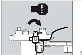
Diverting the fresh-gas flow to the compact breathing system:
