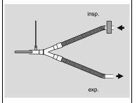
Lateral connections for the sample line support CO2 measurement and help to flush the deadspace between Y-piece and hose adapter.
