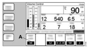
The ventilation settings for the new ventilation mode are automatically derived from the settings of the previous ventilation mode. The corresponding settings (A) in the new ventilation mode are highlighted.
