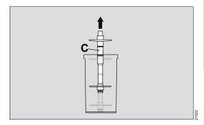
4 If it is necessary to clean the absorber insert (C), remove the absorber insert from the absorber container. Leave the inner and outer sealing rings on the absorber insert.
