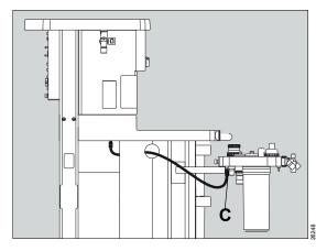
4 Connect the fresh-gas hose (C) to the corresponding connection of the compact breathing system.
