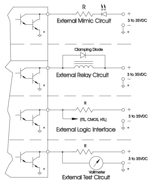
\* Note: All system commons (  $\bigvee\limits_{\sim}$  ) must be tied together.
