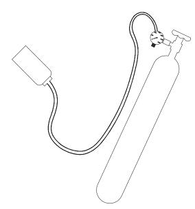
The General Monitors Portable Flow Calibrator is a compact, accurate and safe field calibrator which is used as an alternative to the  $H_2S$  Field Calibrator for sensors located in high humidity environments. The calibrator uses gas bottles filled with known concentrations of  $H_2S$  in dry air. Spare gas bottles are inexpensive and may be returned for refilling. Refer to the table below for the respective part numbers for ordering calibrators and replacement cylinders.
