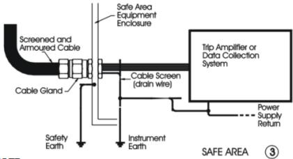
NOTE: Cable Armour connected to Safety Earth via Gland or othervise
