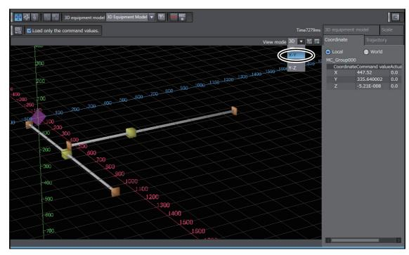
The results of the data trace are displayed in Cartesian coordinates with axis 0 as the X axis and axis 1 as the Y axis.
