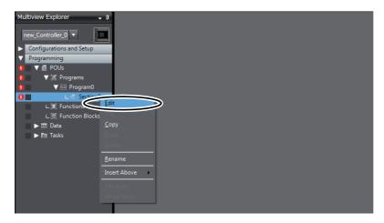
The local variable table and Ladder Editor are displayed in the Edit Pane. From here, you can register local variables and create a ladder diagram.
