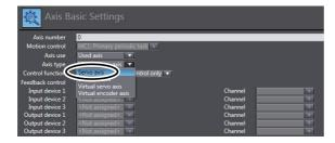
Select thne Servo Drive to use in the *Output device* Box (Node: 1, Device: R88D-1SN01L-ECT).
