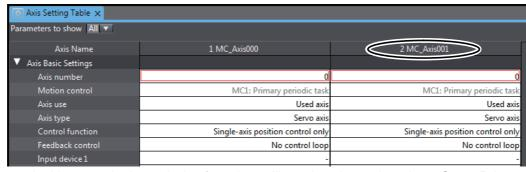
In this state, the input device for axis 1 still needs to be assigned to a Servo Drive.
