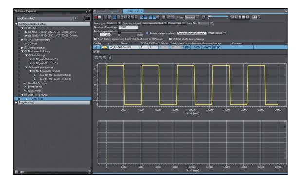
Select the Enable trigger condition Check Box on the DataTrace0 Tab Page and enter the variable to use as the trigger condition. For this example, use Program0.Linear1.Execute.
