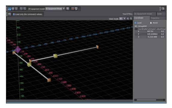
$m{8}$  Click the *View Mode* Box in the 3D Motion Trace Display and select *X-Y* from the list.
