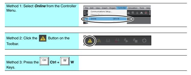
The CPU Unit name is written to the Controller, and the Sysmac Studio goes online with the Controller.
