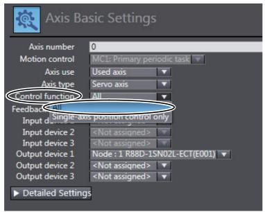
Selecting **All** enables the axis to be used for both single-axis position control and two-axis linear interpolation control.
