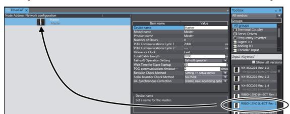
Drag the R88D-1SN01L-ECT from the Toolbox to the master on the EtherCAT Tab Page.
