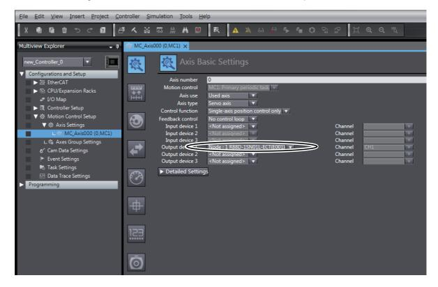
Now, node 1 with device R88D-1SN01L-ECT can be used as an axis in the EtherCAT network configuration.
