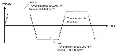
The axis created in Section 3 Setting Up a Single-axis Servo System is axis 0. The axis added in this section is axis 1.
