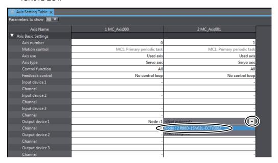
This will assign node 2 and device R88D-1SN01L-ECT as the input device for axis 1.
