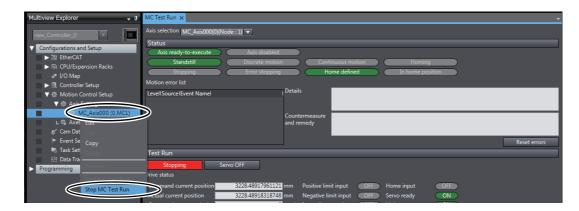
This ends the MC Test Run operation.
