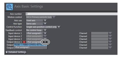
This will assign node 1 and device R88D-1SN01L-ECT as the output device for axis 0.
