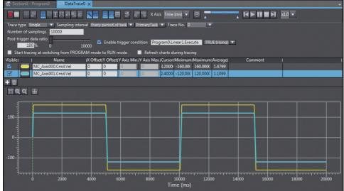
Make sure that the trace results show the same waveform as shown in 4-1 Two-axis Servo System Operation.
