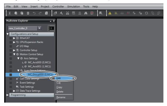
The axes group settings are displayed on the Axes Group Basic Settings Display in the Edit Pane.
