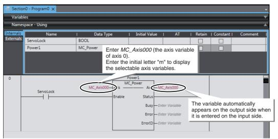
This concludes the creation of the instructions to control turning the Servo ON and OFF.
