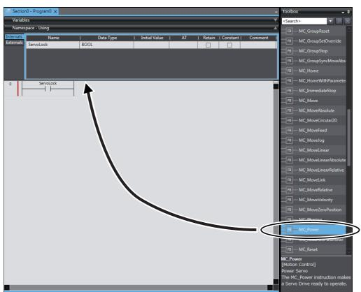
An MC\_Power instruction is inserted to the right of the ServoLock input.
