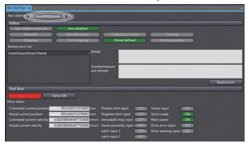
Check to see if the signals turn ON and OFF properly on the monitor screen by turning ON and OFF the sensor connected to each control input signal.
