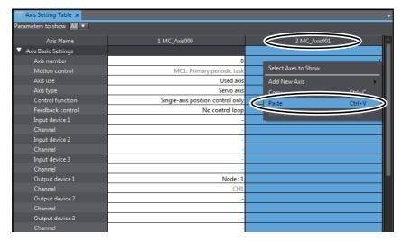
The settings of the axis parameters for axis 0 are copied to axis 1.
