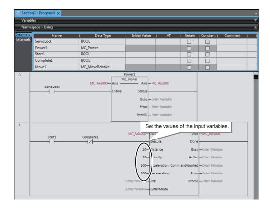
Insert the second MC MoveRelative (Relative Positioning) instruction. Enter Move2 as the instance name, enter the axis variable of axis 0 (MC\_Axis000) for the in-out variable, and enter the values in the following table for the input variables.
