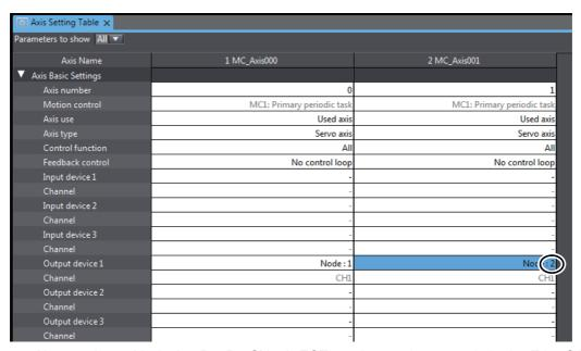
Now, node 2 with device R88D-1SN01L-ECT can be used as an axis in the EtherCAT network configuration.
