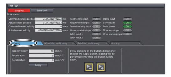
Enter the target velocity, acceleration rate, and deceleration rate, and then click the Apply Button. For this example, set the target velocity to 50.
