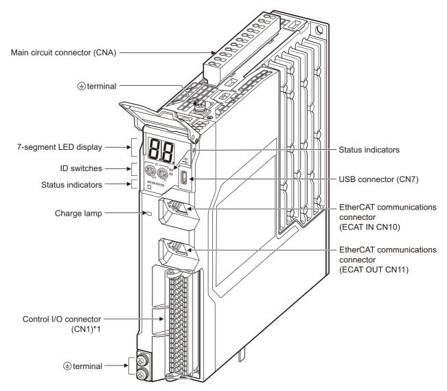
\*1 Control I/O Connector (CN1): Used for command input signals, I/O signals, and as the safety device connector. The short-circuit wire is installed on the safety signals before shipment.
