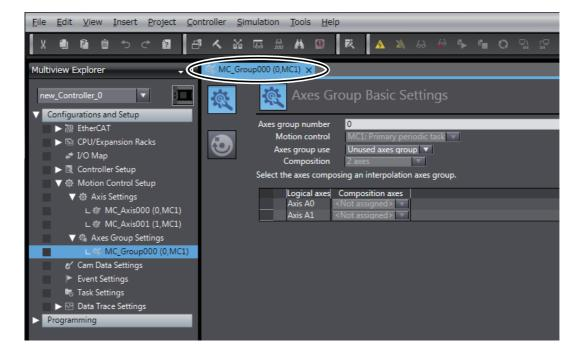
**3** Set the Axes Group Basic Settings for axes group 0 as shown in the following figure.
