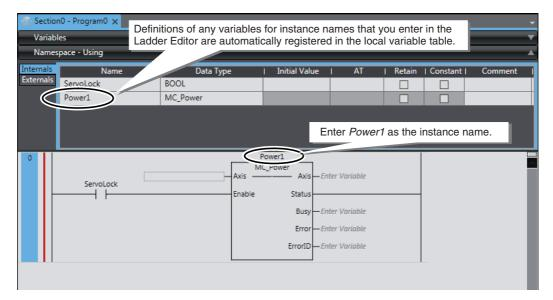
**4** Enter the in-out variable for the Power1 instance.
