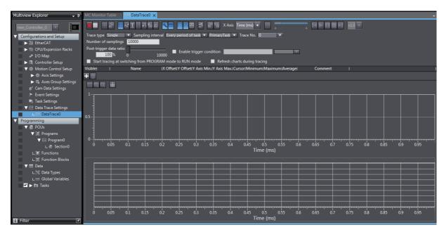
Select the Enable trigger condition Check Box on the DataTrace0 Tab Page and enter the variable to use as the trigger condition. For this example, use *Program0.Move1.Execute*.
