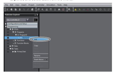
The local variable table and Ladder Editor are displayed in the Edit Pane. From here, you can register local variables and create a ladder diagram.
