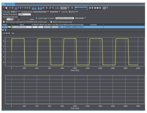
Make sure that the trace results show the same waveform as shown in 3-1 Single-axis Servo System Operation.
