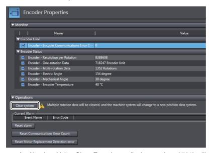
An Absolute Value Clear Error (error display number: 2701) will occur, and a dialog box indicating "Restart the drive to complete the operation."
