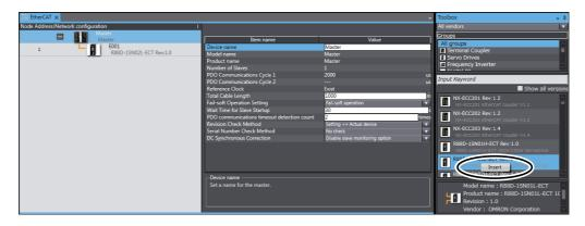
The Servo Drive is added under *E001* with a node address of 2.
