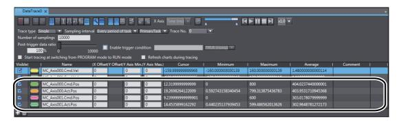
**5** Select the *Enable trigger condition* Check Box on the DataTrace0 Tab Page and enter the *Program0.Linear1.Execute* variable to use as the trigger condition.
