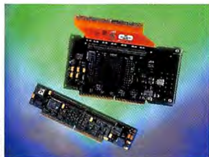
Newer's Maxpowr G3 PDS 240/1MB (top) and Sonnet's Crescendo G3 266/1MB (bottom).
