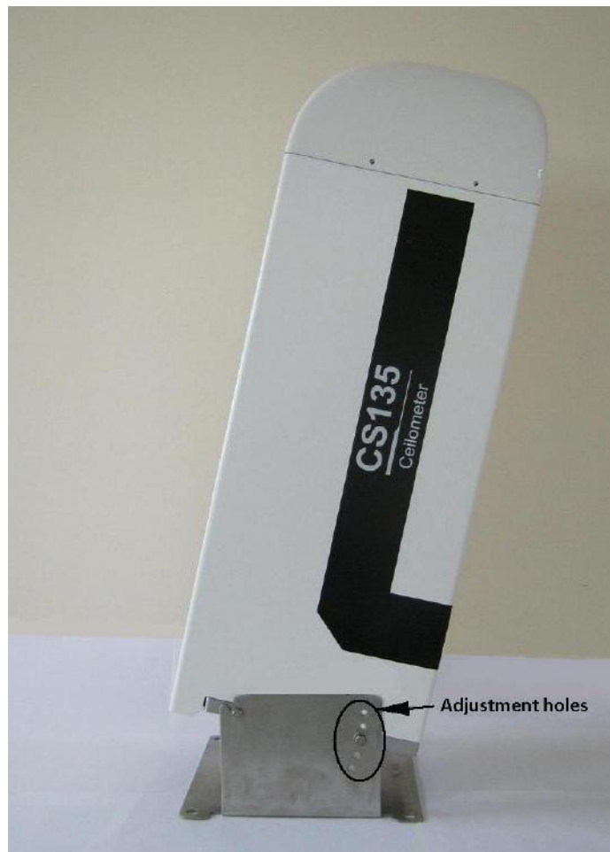
Fig 4.2 Setting the Tilt Angle
