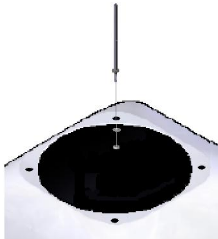
Fig 4.11 Attaching Bird Spikes to the CS135 cowl
