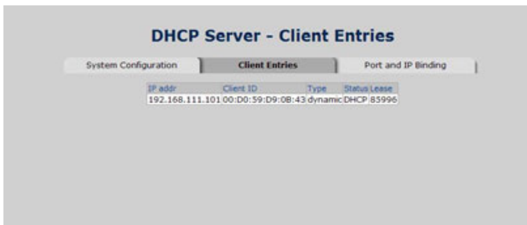
Figure 5-6: DHCP Client Entries interface
