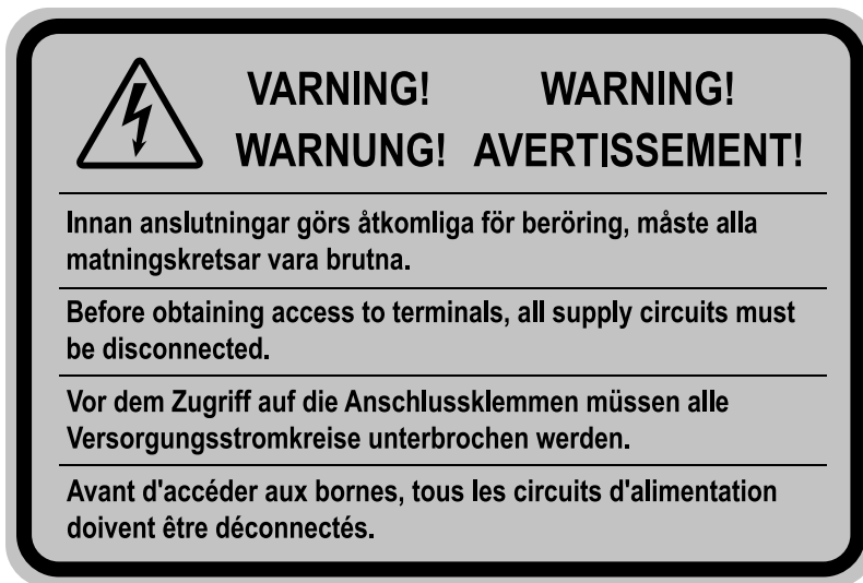
Fig. 1 Disconnect all supply circuits before access to terminals
