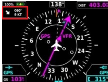
Figure 6-5 HSI Display of Crosswind (Typical Values Shown)
