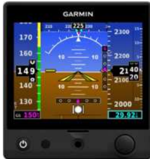
Figure 1-1 G5 Electronic Flight Instrument (Attitude)
