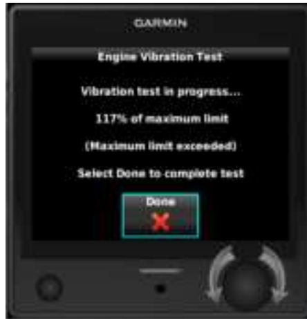
Figure 6-3 Engine Vibration Test Failure Indication
