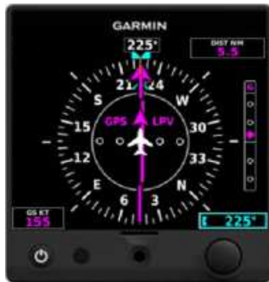
Figure 1-3 G5 Electronic Flight Instrument (DG/HSI)
