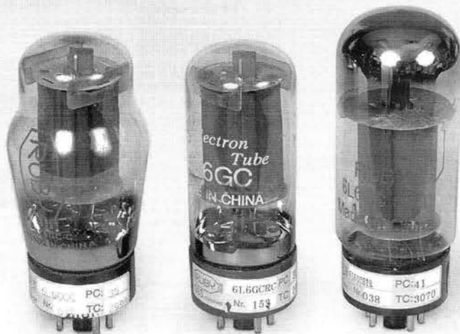
Ruby 6L6 GC-C, 6L6GC-RC and 6L6GC-STR (1990s)
