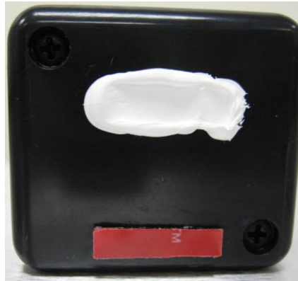
Figure 5 - Adding Bonding Adhesive to the ELS Sensor Module and attach to Battery Case
