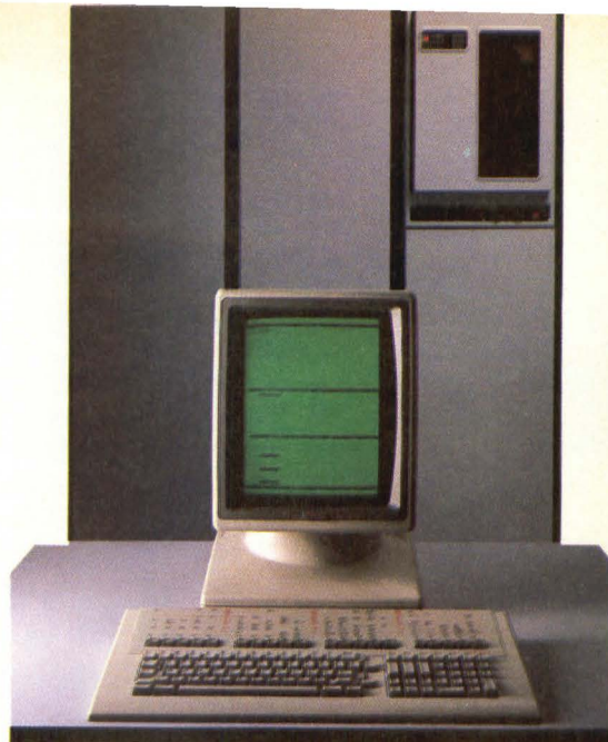
The Rational R1000 software development system, in addition to a specialized processor, has a full-screen, multiple window terminal.
