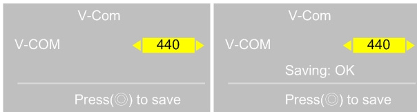
(Visual Adjust and control the Voltage level)
