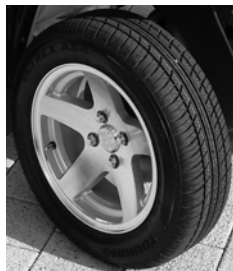
Aluminum Wheel (12-inch / 14-inch) 95 ft. lbs. (128 Nm)
