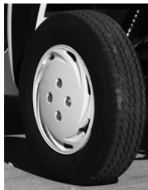
Steel Wheel (12-inch / 13-inch) 65 ft. lbs. (88 Nm)
