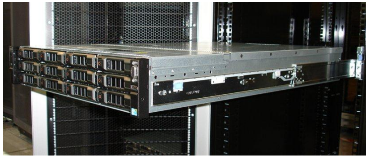
Figure 8. R515 Mounted in B3 Sliding Rails
