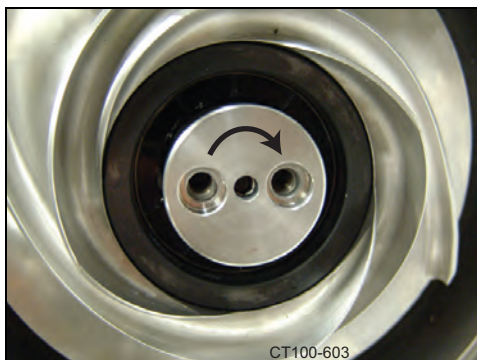
Figure 65 - Rotate inner magnet assembly
