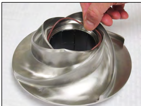
Figure 43 - Install front impeller o-ring
