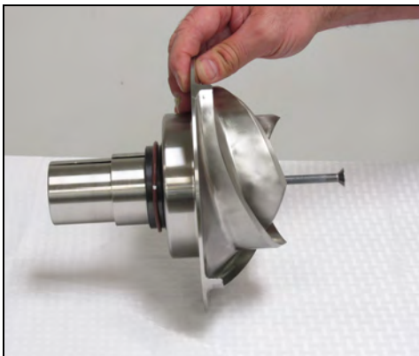
Figure 55 - Hold shaft in place
