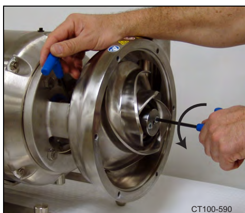
Figure 14 - Remove mounting bolts
