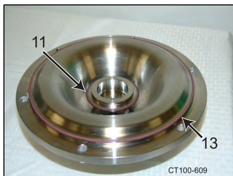
Figure 73 - O-rings installed on nose and cover
