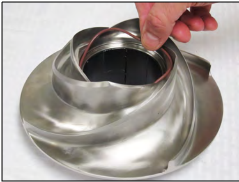
Figure 28 - Remove front impeller o-ring
