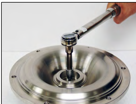
Figure 72 - Torque nose bolt
