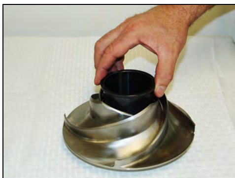
Figure 45 - Place impeller on the tool
