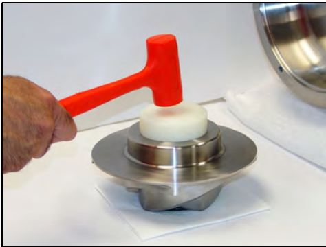
Figure 25 - Tool flush with impeller face
