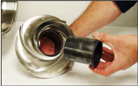
Figure 21 - Remove canister from impeller
