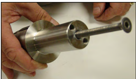
Figure 51 - Leave screw protruding from shaft
