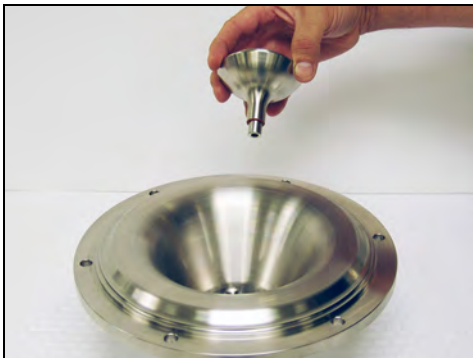
Figure 70 - Install nose onto cover
