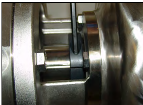
Figure 64 - Place Allen wrench in bolt head to keep shaft from rotating
