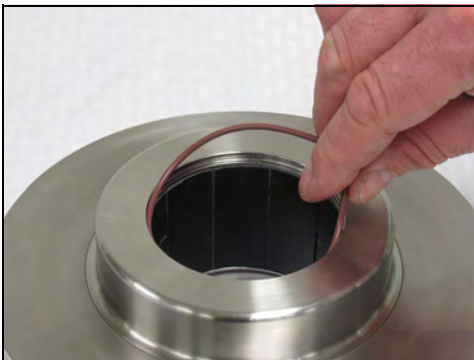
Figure 27 - Remove rear impeller o-ring
