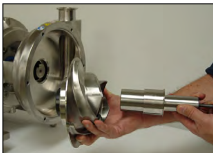
Figure 19 - Remove shaft from impeller assembly
