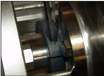
Figure 58 - Align motor shaft collar
