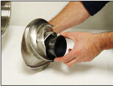
Figure 52 - Install canister into impeller
