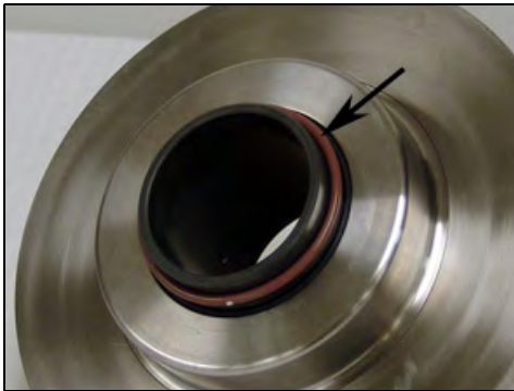
Figure 53 - Install o-ring onto canister
