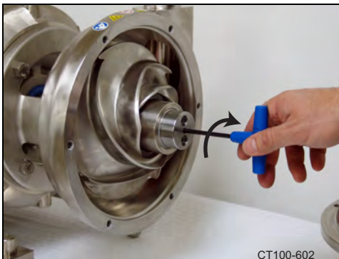
Figure 62 - Screw in magnet jack screw
