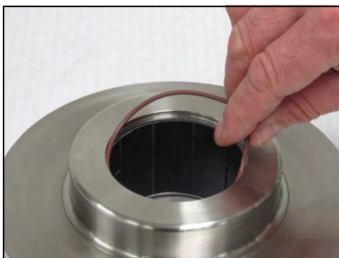
Figure 41 - Insert rear impeller o-ring
