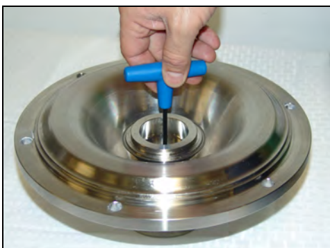
Figure 31 - Unscrew nose bolt
