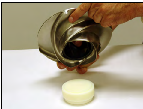
Figure 46 - Place impeller on the tool
