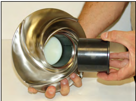
Figure 26 - Remove bushing from impeller
