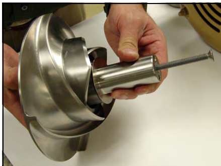
Figure 54 - Insert shaft in canister
