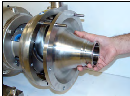
Figure 11 - Install guide rods and remove cover
