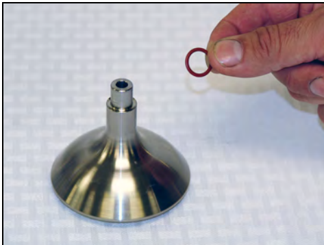
Figure 68 - Install nose-to-cover o-ring
