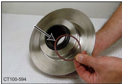
Figure 20 - Remove canister-to-casing o-ring
