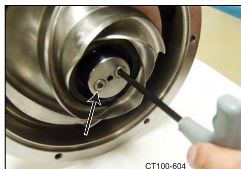
Figure 66 - Tighten inner magnet assembly screws
