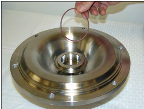
Figure 30 - Remove nose-to-canister o-ring from nose
