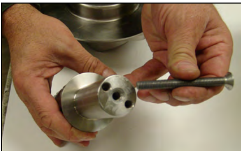
Figure 50 - Thread magnet jack screw
