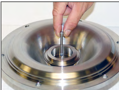
Figure 71 - Install nose bolt
