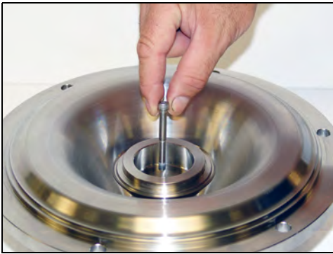
Figure 32 - Remove nose bolt
