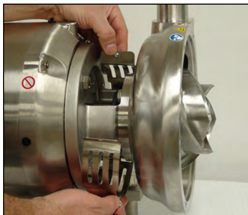
Figure 13 - Remove shaft guard
