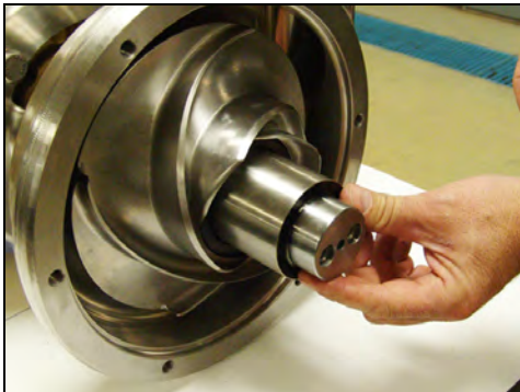
Figure 61 - Center the magnet assembly
