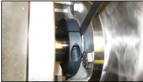
Figure 57 - Position motor shaft
