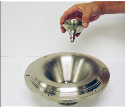
Figure 33 - Remove nose from cover
