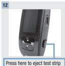
Remove and discard the used test strip by pulling the test strip out of the meter or by pushing the test strip ejector on the side of the meter.
