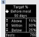
The **Target** % appears (for the **Before meal** example). The number of total tests included in the Target % appears at the bottom of the display.
