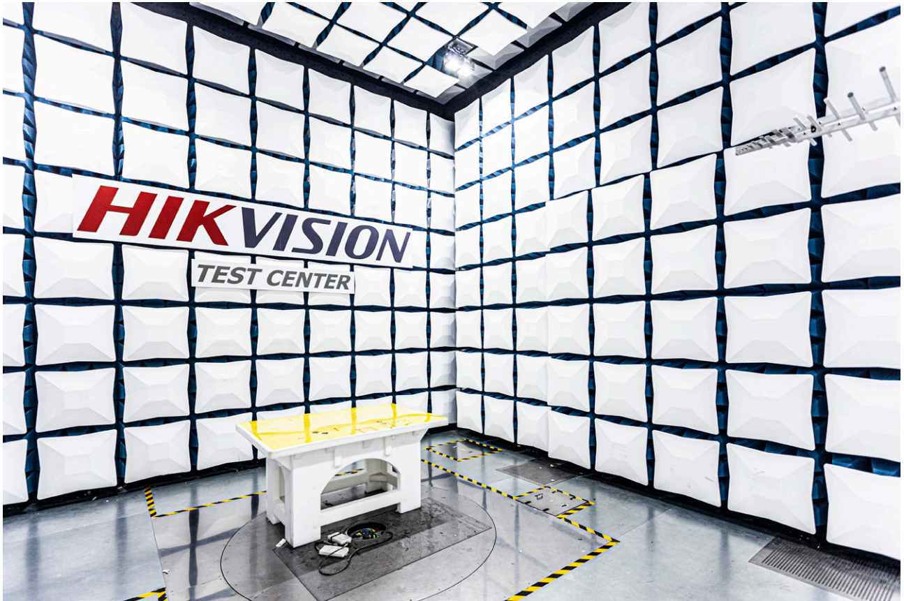
EMC Testing Anechoic Chamber
