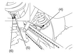
(4) rebound damping adjuster(6) reference mark(5) punch mark
