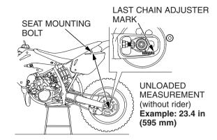
3. Measure the *loaded with rider* dimension. Remove the workstand. With two helpers available, sit as far forward as possible on your CR's seat, wearing your riding apparel. Ask one helper to steady your CR perfectly upright so you can put both feet on the pegs. Bounce your weight on the seat a couple of times to help the suspension overcome any situation and settle to a good reference point.
