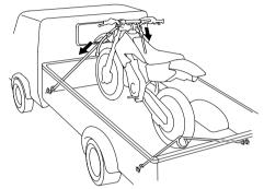
To secure your CR, brace the front wheel against the front of the truck bed or trailer rail. Attach the lower ends of two straps to the tie-down hooks on your vehicle. Attach the upper ends of the straps to the handlebar (one on the right side, the other on the left), close to the fork.
