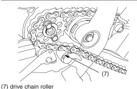
8. Check the driven sprocket nut torque values after each race. 24 lbf·ft (32 N·m, 3.3 kgf·m)
