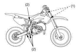
(1) steering head bearings(2) suspension pivot points
