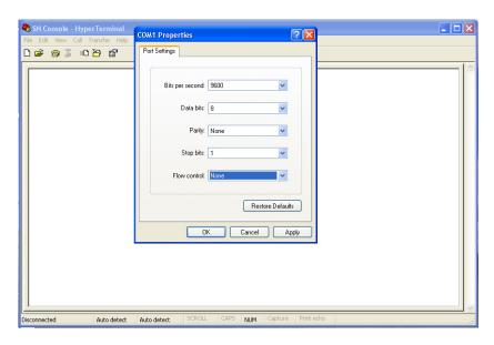
Bits per Second: **115200**, Data Bits: **8**, Parity: **None**, Stop bits: **1**, Flow Control: **None**.
