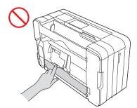
DO NOT carry the machine by holding the scanner cover, the Jam Clear Cover, the manual feed slot cover, or the control panel. Doing this may cause the machine to slip out of your hands. Carry the machine by sliding your hands into the handhold indentations located on each side of the machine.
