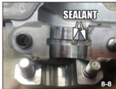
Sealant Plugging Lubrication Channel
