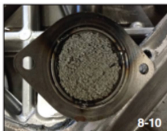
Oil Screen Plugged
