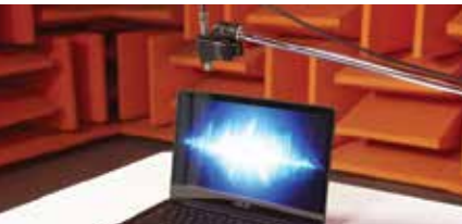
Noise and Audio Test Laptops undergo fan, hard drive, and power-supply noise tests to ensure the quietest performance possible.
