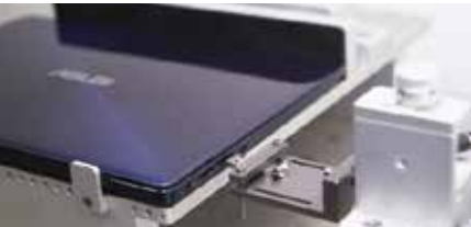
Port Test Port tests ensure that contacts and plugs are durable even in environments where devices are frequently connected and disconnected.
