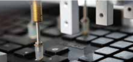
Keyboard Test To ensure ultimate keyboard durability, specially designed ASUS robots test individual keys with millions of keystrokes.
