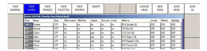
Channels can be added using the Insert soft button and deleted using the Remove Button (press twice to Remove).
