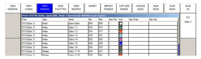
This view defines the ranges for channels that utilise specific values to access functions such as colour and gobo wheels, shutter channels and control channels. Ranges can be set up at any time regardless of whether heads of the type have been patched and the range data becomes immediately available. If the head has been patched then you can capture the minimum and maximum value fields from the programmer.
