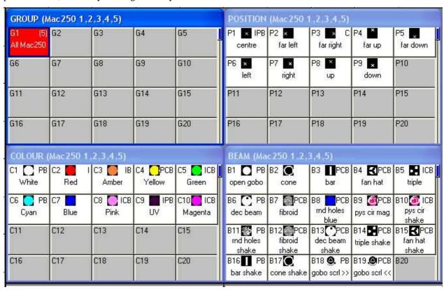
In the Colour Window there is a COL MIX soft button which gives access to libraries of pre-programmed colours. Pressing the COL MIX soft button toggles between the normal palette view and the colour mixing view. In the colour mixing view you can select a colour using the touch screen. The COL TYPE soft button enables the user to choose between the default colour library, the Lee colour library or the Rosco colour library.
