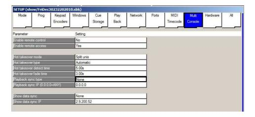
In manual mode, when MagicQ determines that it should take over a universe it will load a snapshot of the last data from that universe into its Programmer. Thus the universe will be completely controlled from
