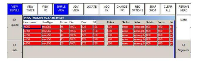
In the Channel Times and Channel View windows you have a choice of a Simple View or an Advanced View. The Simple View is sufficient for most programming – it enables modifications of fade times on a per attribute type basis and modifications of each programmed FX. The Advanced View enables fade times and FX parameters to be set up on a per channel basis.
