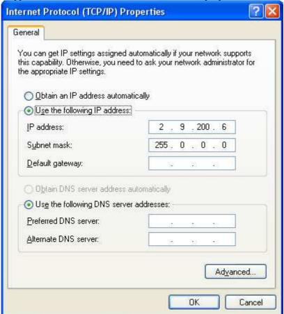
You will be presented with a radio button choice between "Obtain an IP address automatically" and "Use the following IP address". Choose "Use the following IP address". Enter the IP address (e.g. 192.9.200.1) and the subnet mask (255.255.255.0). The default gateway address can generally be left blank. Click ok. Older Windows systems will request a restart - select "restart now".
