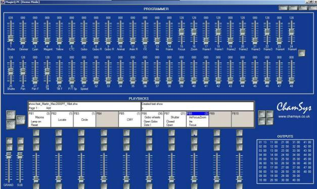
The Playback faders are automatically set up with some useful functions including Macros for Lamp On, Reset and Lamp Off, Locate and Movement, Colour, Gobo and Strobe tests.
