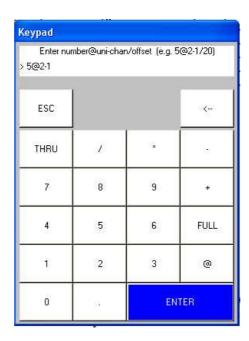
To patch a head at a specific address use @. For example to patch 10 dimmers at DMX address 20 key in 10@20. To patch to the  $2^{nd}$  universe use 10@2-20. To patch at the first free address on a universe other than the first universe use +, e.g. for the second universe use 10@+2-1.
