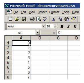
From v1.6.0.7 dimmer curves can have 16bit values (0..66535) instead of just (0..255). If any value in theuser dimmer curve file is over 255 then 16bit is assumed.
