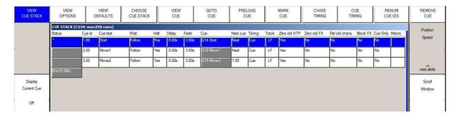
The status field indicates the current status of the Cue in the Cue Stack. If the Cue is active (i.e. it is in the process of execution) then the field indicates a % complete and the entire cue is coloured red.
