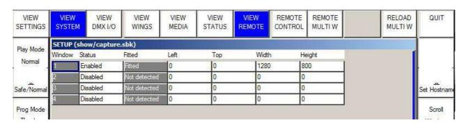
The remote control function is accessed through the new View Remote option in the View System view of the Setup Window. To control another MagicQ press the Remote Control soft button. MagicQ then presents a list of all the other MagicQ consoles / MagicQ PC systems it can find on the network and you can choose which one you wish to control.
