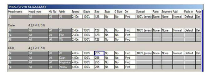
When viewing and editing multiple FX in the Programmer Window or Cue Window the encoders A,B,C,D,X and Y affect only the FX that the cursor is placed over. Prior to v1.3.2.4 they always affected all FX in the Programmer/Cue. When a new FX is added the encoders automatically default to controlling the parameters of the new FX.
