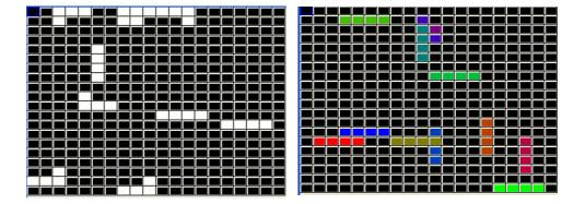
Bat'n'Ball – enables simple bat and ban game on the grid. The bats are controlled by FX Parameters 2 and 3. The game starts when one of the bats is moved. Other bitmap layers can be combined with this to make a background for the playing field.
