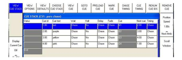
In Theatre Modes the default timing is Cue Timing – individual Fade times on each step with GO stepping from one step to the next.
