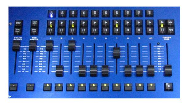
The playback area also contains a Grand Master, a Sub Master, Page Select buttons and a Manual Playback for taking control of Cue Stacks.
