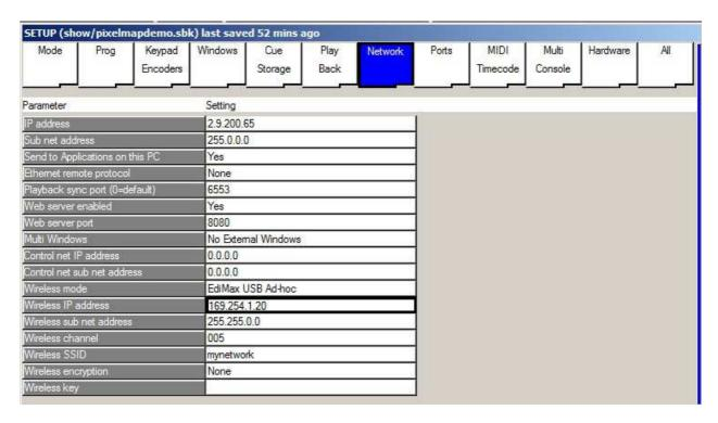
The Wireless channel defaults to 0 indicating that the Edimax device will automatically pick a channel. If you wish to force use of a particular channel enter a number between 1 and 11.
