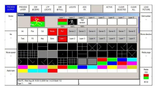
MagicQ asks the user to specify the number of layers required and will patch that number of layers (generic bitmapfx2 heads). The layers will be named according to the grid that is selected in the Outputs Window. MagicQ uses head numbers above the other patched fixtures
