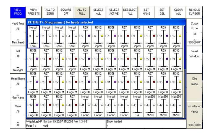
The SQUARE OFF soft button enables fast programming of intensities. Using the touch screen select the channels you wish to have at full and at zero – but don't bother being exactly accurate with the level of the selection. Pressing SQUARE OFF finishes the job by setting all channels that are less than 50% to 0 whilst setting channels above 50% to full.
