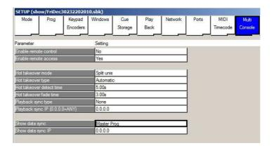
On each of the slave consoles set the "Show data sync type" option to "Slave Prog" and set the "Show data sync IP" to the IP address of the master show console.
