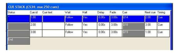
The timing mode can be changed, so that the Cues play back in a theatre style using the GO / STOP buttons. Select the VIEW OPTIONS view and press the CUE TIMING and CHASE TIMING soft buttons to modify the timing mode.
