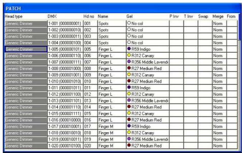
The gel field uses gel numbers. For Lee colours enter the gel number directly (e.g. 181 for Lee 181). For Rosco colours enter the gel number preceded by dot (e.g. .14 for Rosco 14). For no colour enter 0. If you would prefer to use colour names rather than gel numbers then simply enter the colour name.
