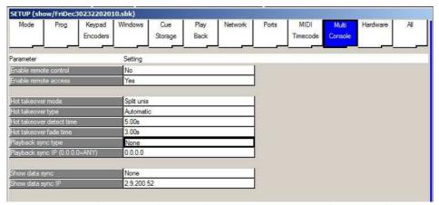
In manual mode, when MagicQ determines that it should take over a universe it will load a snapshot of the last data from that universe into its Programmer. Thus the universe will be completely controlled from within the Programmer and not from the Playbacks. The operator can then set up the playbacks as they wish and then clear the programmer to change to this new look. Clearing the programmer with time enables the operator to specify a fade time to the new look.
