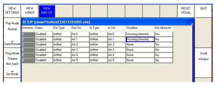
If you are using WYWISYG on the same PC as MagicQ then set the Visualiser to WYSIWYG (same PC) – otherwise, set it to WYSIWYG (remote). When connecting to WYSIWYG using a MagicQ console, always use WYSIWYG (remote).
