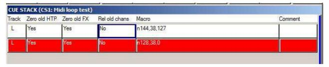
MIDI note commands are 3 bytes long, consisting of the command (note on / note off) byte, followed by the note and then the velocity
