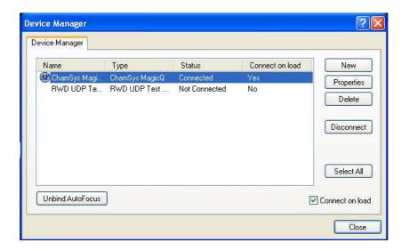
The universes in WYSIWYG must be bound to the ChamSys MagicQ device in order for communication to occur with MagicQ.
