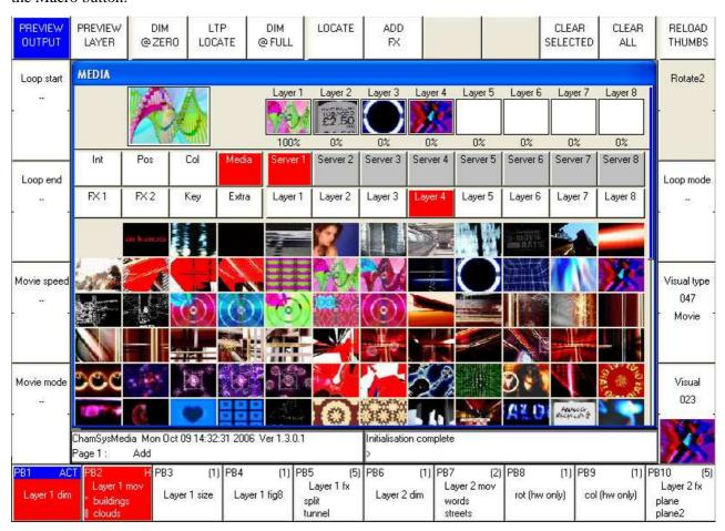
In addition, there is a Live Preview window, which shows the output of the media server, or the output of each of the layers. This is transferred is real time from the media server – so that you can see exactly what the media server is playing. This is particularly useful in situations with many media servers, or media servers that are remote from the control position.
