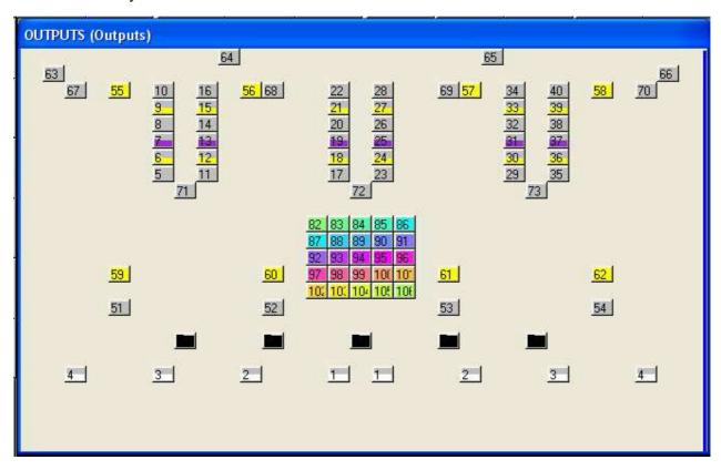
In the Outputs Window, select View Plan and View Hd Nos. Press Grid Size and enter a matrix size for your lighting rig - e.g. 30/20 gives a 30 by 20 grid.
