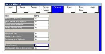
Cues can be set to time code by changing the Halt field in the Cue Stack window (double click on it or press SHIFT + ENTER.
