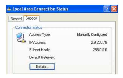
To determine the IP address of the media server on Windows XP machines, load the Control Panel, and open the Network Connections screen. Double click on the network connection, choose the support tab, and the IP Address is displayed.
