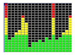
Ramp Horiz and Ramp Vert – these perform a ramp across the entire grid in the horizontal or vertical directions. FX P1 parameter controls the speed, FX P2 controls the crossfade and FX P3 controls the width.
