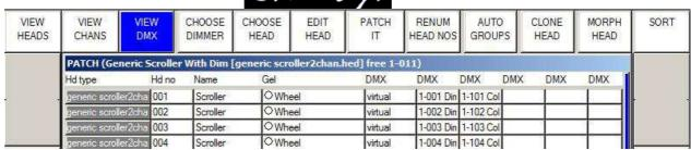
To use this support, patch a Generic Scroller With Dim. This will appear in the View Heads with the DMX address marked as "virtual" and any DMX address you specified when you patched it will be ignored. Change to the View DMX view and specify in the appropriate DMX columns the DMX address of the dimmer and the scroller.
