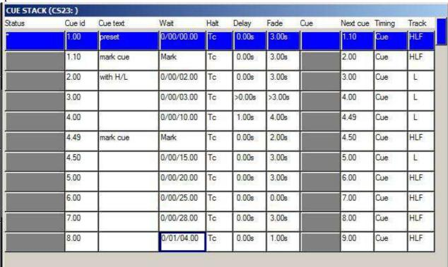
When a Cue Stack that contains time code cues is activated the time code takes control of the Cue Stack and each Cue executes at the time code specified. For Internally generated time code, activating the Cue Stack starts the time code at 0/0/0. For external time code the time code will be read from the external module.
