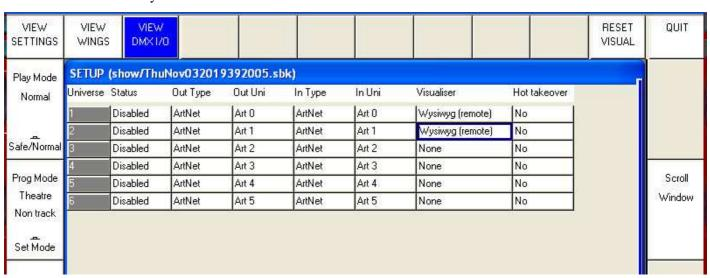
If you are using the Visualiser on the same PC as MagicQ then set the Visualiser Type to (same PC) – otherwise, set it to (remote). When connecting to WYSIWYG using a MagicQ console, always use WYSIWYG (remote).
