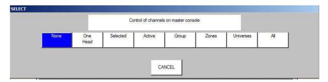
The options allow control of a single head (One Head) all the way through the whole rig (All) by this show slave.
