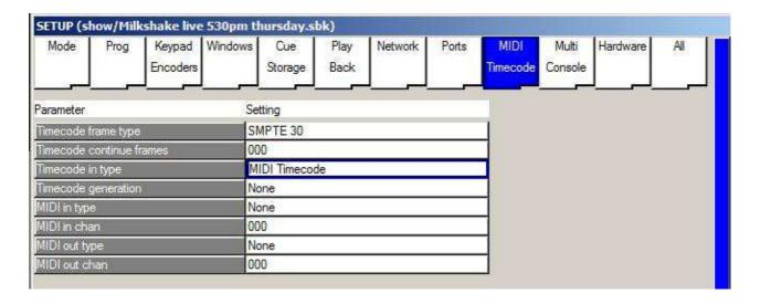
Enable timecode receive in the Timecode In Type field, and choose between SMPTE and MIDI Timecode.
