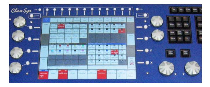
The function of the rotary encoders also changes according to the active window with the current function being displayed adjacent to the encoder.
