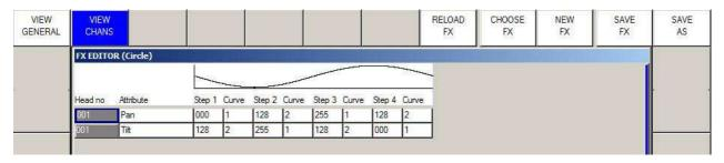
FX that have been recorded in a show, but that have not been stored onto the console can be extracted from the show by including the Cue that uses the FX. This will bring the FX into the FX Editor, and it can then be saved on the console.
