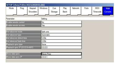
There are hot keys on the slave consoles to enable and disable the show sync (as set up in Setup, View Settings, Multi Console). Hold the left and right cursor keys and press '+' to enable the show sync and hold left and right cursor keys and press '-' to disable the show sync.
