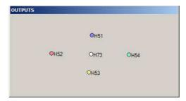
The movement view shows the relative positions of heads in terms of pan and tilt range on a 2D map. It also shows the current colour of the heads. This enables previewing of FX and relative positions without the lighting rig. Press the VIEW CHANS, VIEW DMX, VIEW MOVE soft buttons.
