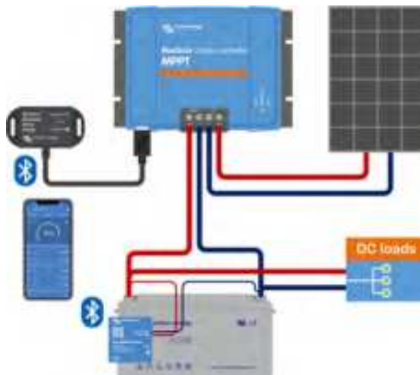
Example of a VE.Smart Network of a Smart Battery Sense and a solar charger
