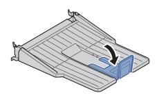
Install the rear tray on the rear of the machine.
