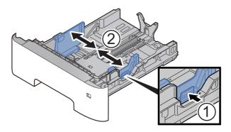
2 Adjust the paper length guide to the paper size required. Press the paper length adjusting tab and slide the guides to the A6 size.
