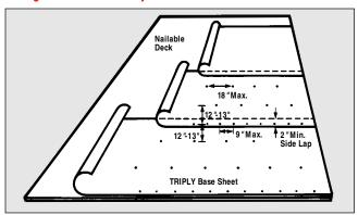
All nailing must be done through flat metal caps or acceptable nails with 1 inch square or round metal caps. The proper nail or fastener must be selected in accordance with the recommendations of the deck manufacturer or as recommended for specific type decks in this catalog. The fastener used must have a minimum withdrawal strength of 40 pounds.
