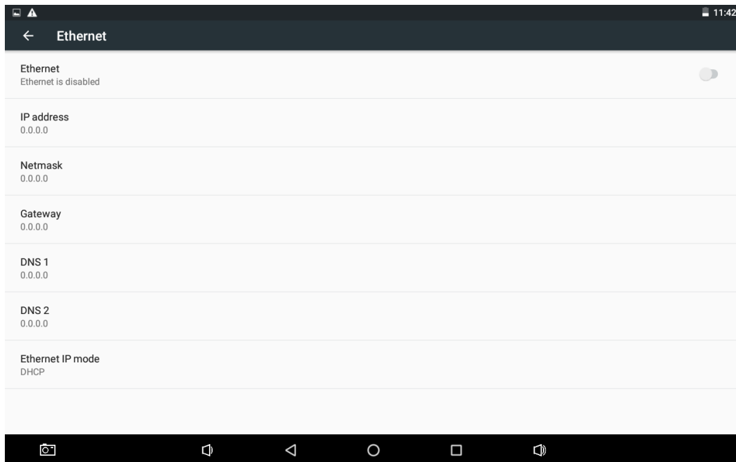
Figure 19: Connecting to Ethernet – Enabling Ethernet
