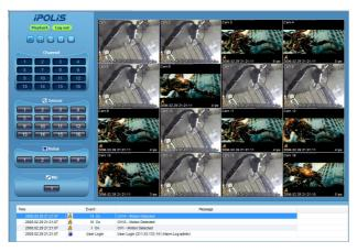
Input User ID와 Password at Login page, and move to Monitor page if it is authorized normally. At Monitor page, it can monitor real-time camera image connected to product or use PTZ camera control, Relay and microphone function connected according to user authority.
