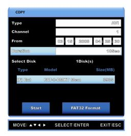
It is to Copy a part of one channel selected to USB memory or HDD.
