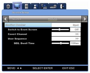
Basic monitor is used for all functions of DVR like Menu setup, Live images (16 divisions) and Playback, and Spot monitor can be used for two functions of Single channel live image and Event pop-up image.
