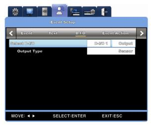
D-I/O is Port able to use digital Input & Output simultaneously. It has 12 Digital Input & Output.
