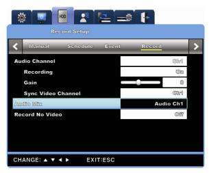
Select Audio to use from Live image. In case of All setup, all input audio is out in mixed. And when selecting specific audio, it is out bony selected channel unconditionally whatever any channel is selected.
