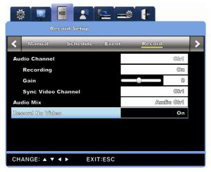
It sets whether it records the input image that has fault or the channel delete image intentionally or not. When it sets to On, it records the channel that video does not input also, and it does not record the channel video is not input when it sets to Off.
